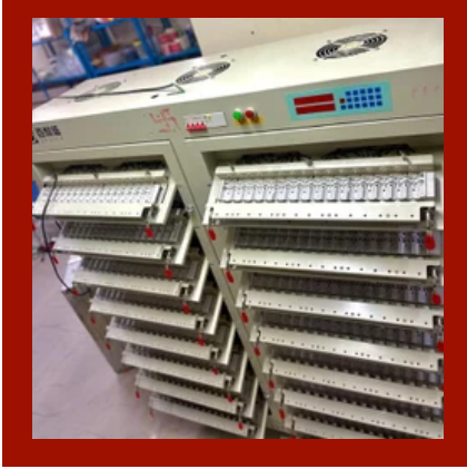
512 Channels 5V 3A 5A Lithium Battery Grading Machine for Cylindrical Cell Testing
