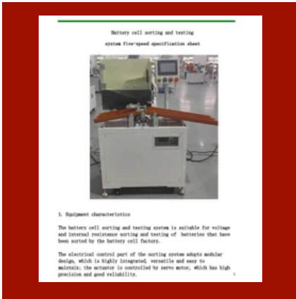
Battery cell sorting and testing system
